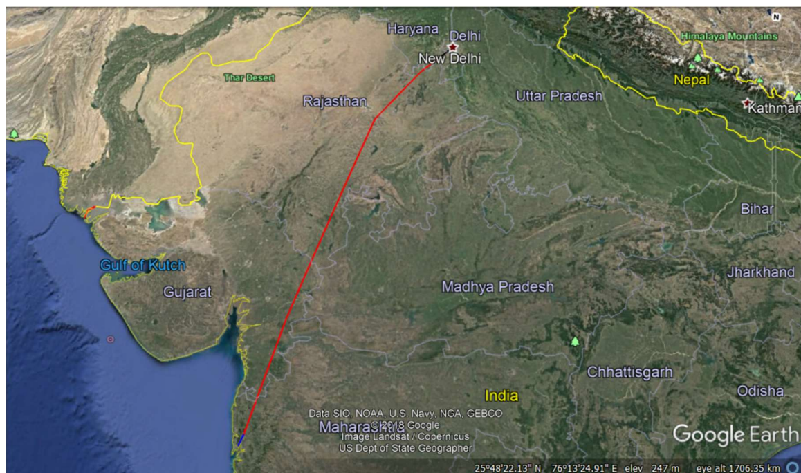
Figure 1: Map of the proposed route between New Delhi and Mumbai, India. The red line represents the aboveground track, whilst the blue and black lines represent the underground tracks. Although not shown in this map, the turns in the track will have minimum radii of 2.5 km to minimise experienced g-forces by passengers.
